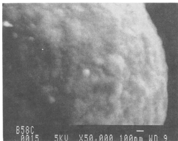
Fig. 25. SEM micrograph of the surface of a coacervated zirconia particle [91].
